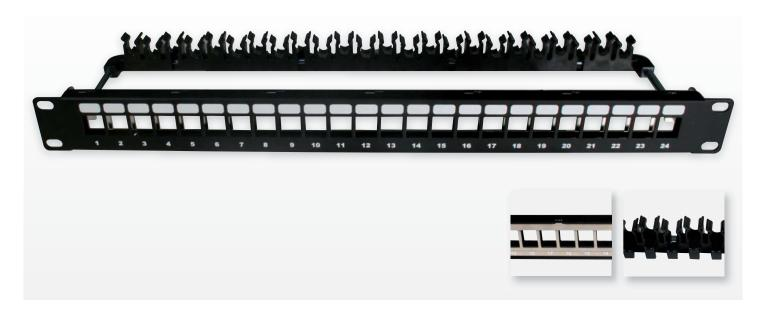
Category 6<sub>A</sub> unloaded panels accept category 6A 10G screened jacks and are supplied with cable management bar. Plastic clips are included on the rear management bar to handle rear cable management easily. Identification number are included both on front and rear of panel
